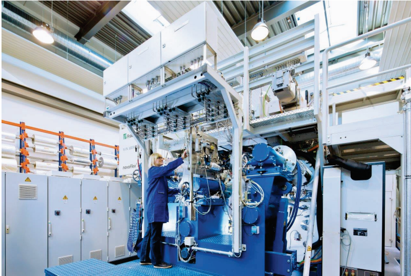
novoflex® 600 roll-to-roll pilot strip coater, on which the new process for the deposition of columnar silicon layers © Fraunhofer FEP
