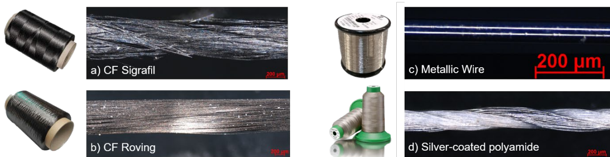
Figure 3: Materials for the sensor yarns and microscopic view; modified carbon fibre yarn (Sigrafil) (a); carbon fibre roving (CF1K) (b); Isohm metallic wire (Isohm) (c); Silver tech 120 (ST120) (d).
