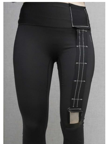
The textile sensor above the knee is connected to an antenna embedded in the waistband. Together, they form a circuit that can be used to measure movement.
