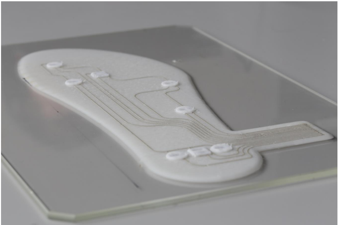
The personalized insole with integrated sensors can measure the pressure of the sole in the shoe during different activities.
