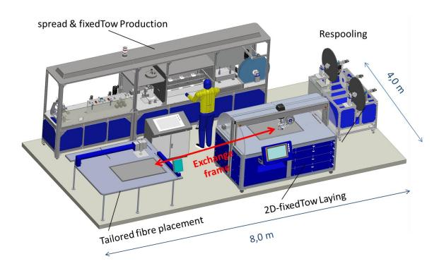
Combine FixedTow laying with with tailored fibre placement for simplified and optimized preforming: Novel Tailored fixedTow Placement Machine for fast results and ease of use.
