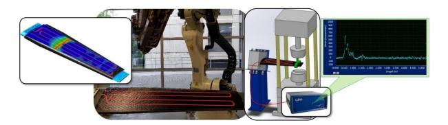
A validated optimized methodology for design of passive shape adaptive structures. This 1:1 scale 3D part was embedded with fiber-optic sensors and manufactured using Automated Fiber Placement robot.
