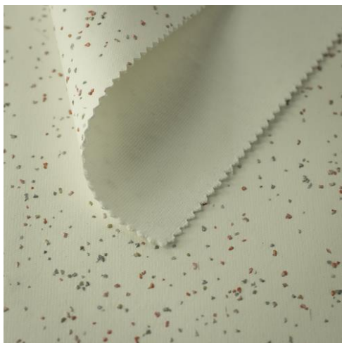
B.Cork™ coating on a cotton base
